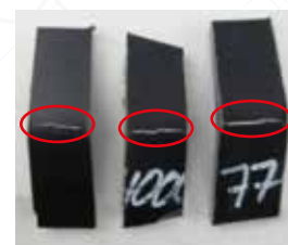
Figure 4: Front view of the three samples from the original equipment manufacturer after the bending test. Cracks visible on all samples.
