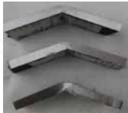
Figure 1: Side view of the three GRANIT samples after the bending test. No cracks visible.
