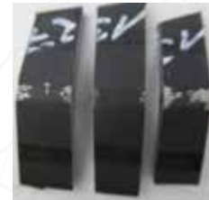
Figure 2: Front view of the three GRANIT samples after the bending test. No cracks visible.
