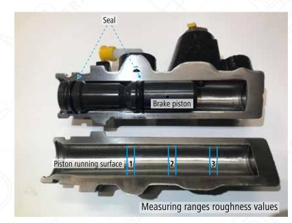
Figure 3: Interior view of the cylinder. Ranges of measurements for the roughness values on the functional surfaces of the two piston seals.
