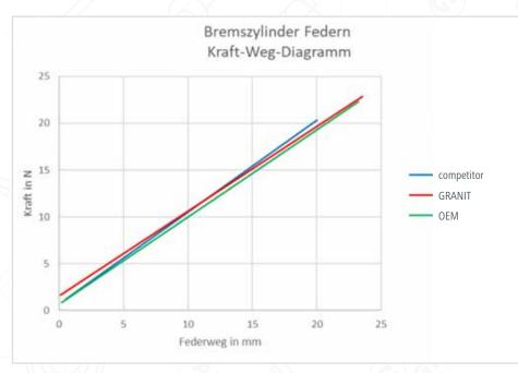
Figure 5: Determination of the spring force.
