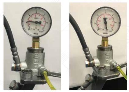
Figure 7 and 8: Possible pressure build-up before venting and after venting.
