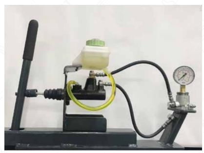
The mounting of the MBC and the assembly of the brake hoses could be done without any problems. The threaded holes provided for attaching the brake hoses were made professionally and cleanly by all manufacturers. The subsequent venting of the three MBCs was also carried out smoothly. All three MBCs are in accordance with the function.
